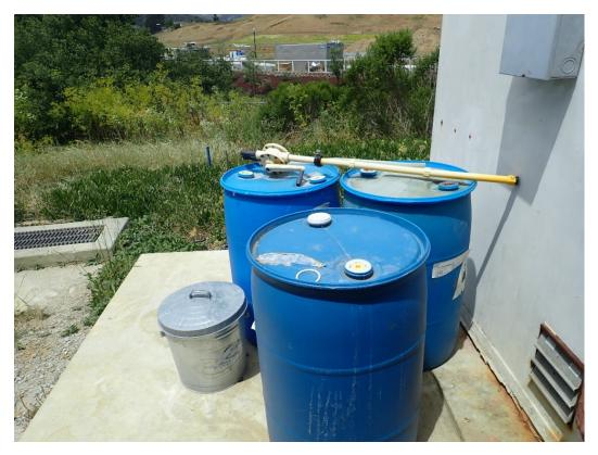
Photo 25 : Full 55 gallon drums stored outside without secondary containment.
