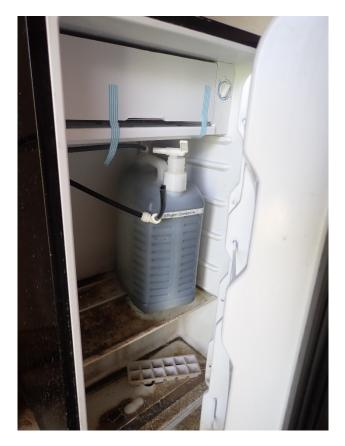
Photo 17 : Refrigerator containing composite sample container.
